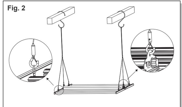
2. Secure both ends of the fixture to the three eyehooks of the cables, as shown. (Fig. 2)
