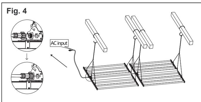
4. Connect the power cord to the fixture, as shown. Make electrical connections; the fixture is rated from 120-277VAC. (Fig. 4)
